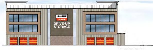
EAST ELEVATION: BUILDING B Scale: 1" = 20'
